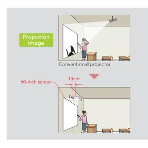
The Ultra Short Throw series has a remarkable short-focus lens that presents 60-inch screen size from a mere distance of 13cm. The short throw eliminate shadows that often appear on-screen and keeps the light from the light source away from the presenter's eyes.
